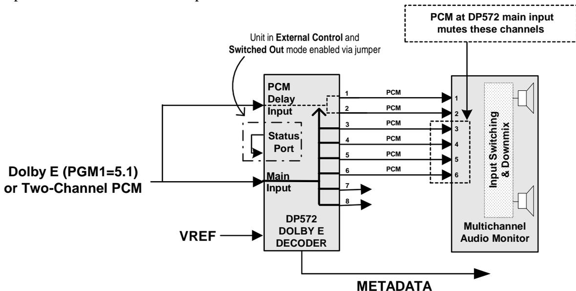
In the figure above, the DP572's eight outputs are shown individually only for clarity. The eight output channels actually reside on four AES pairs.
