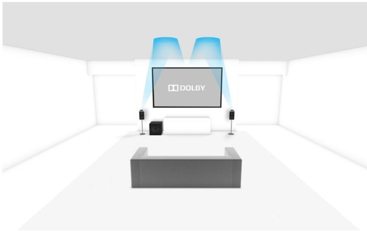
Figure 1: A traditional 2.1 speaker layout with two listener-level speakers and two Dolby Atmos enabled speakers (2.1.2)
