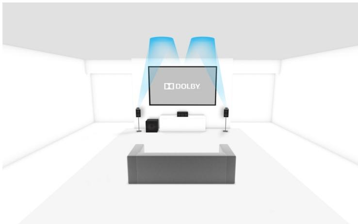
Figure 2: A traditional 3.1 speaker layout with three listener-level speakers in addition to two Dolby Atmos enabled speakers (3.1.2)
