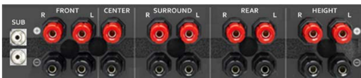
Figure 7: Rear panel of a 7.2.2 AVR. Height speaker connections are on the right.
