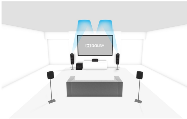
Figure 6: A traditional 5.1 speaker layout with two Dolby Atmos enabled speakers (5.1.2).
