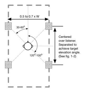
Figure 4: Top view, height (overhead) speaker positioning.
