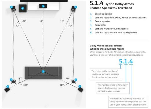
Speaker placement for 5.1.4 hybrid setup
