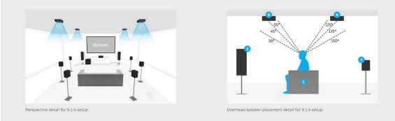
Figure 25: Standard 9.1.4 setup with overhead speakers.
