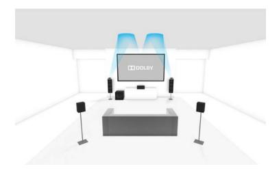
Figure 10: A traditional 5.1 speaker layout with two Dolby Atmos enabled speakers (5.1.2).
