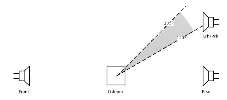
Figure 36: Side view of left rear height and right rear height speaker placement.
