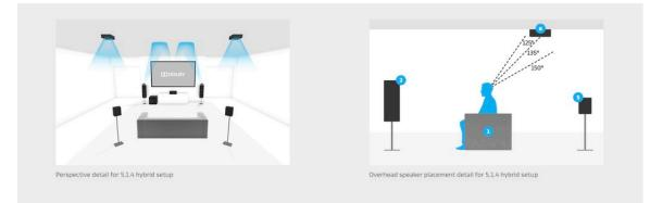
Figure 16: Hybrid 5.1.4 setup with front Dolby Atmos enabled speakers and rear overhead speakers.
