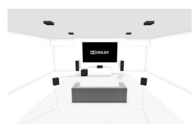
Figure 9: A traditional 5.1 speaker layout with four overhead speakers (5.1.4).
