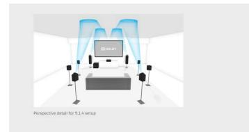
Figure 26: Standard 9.1.4 setup with Dolby Atmos enabled speakers.
