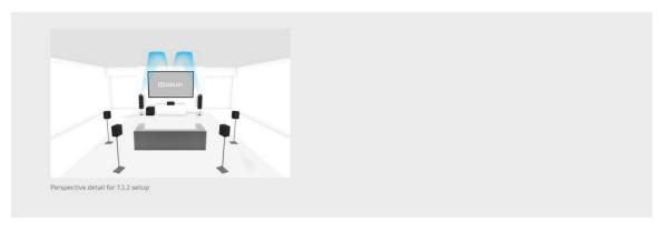
Figure 18: Standard 7.1.2 setup with Dolby Atmos enabled speakers.
