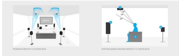
Figure 21: Hybrid 7.1.4 setup with rear Dolby Atmos enabled speakers and front overhead speakers.
