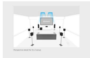
Figure 24: Standard 9.1.2 setup with Dolby Atmos enabled speakers.
