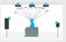
Overhead speaker placement detail for 9.1.6 setup
