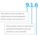
This refers to how many overhead or Dolby Atmos enabled speakers you can use in your Dolby Atmos capable setup.
