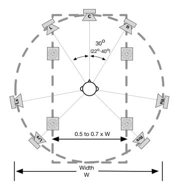
Figure 3: Top view, listener-level and height (overhead) speakers in a 7.1.4 configuration.
