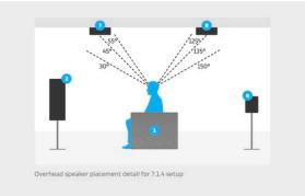
Figure 19: Standard 7.1.4 setup with overhead speakers.
