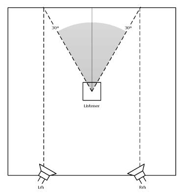
Figure 37: Top view of left rear height and right rear heigh t speaker placement.
