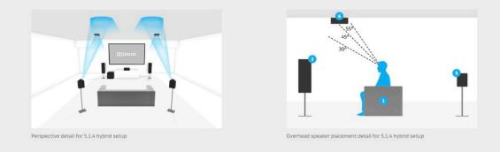
Figure 15: Hybrid 5.1.4 setup with rear Dolby Atmos enabled speakers and front overhead speakers.
