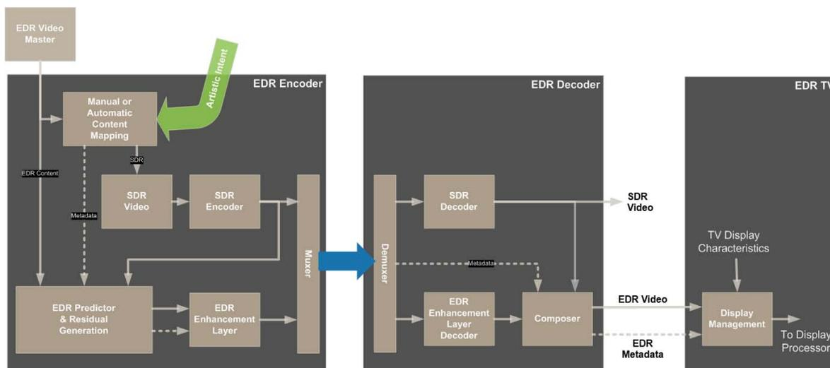
Figure 11 – The EDR Dual Layer Codec
