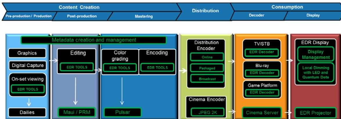
Figure 10 - Off-line EDR System Architecture / Workflow
