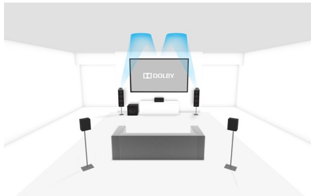
Figure 9: A traditional 5.1 speaker layout with five listener-level speakers and two Dolby Atmos enabled speakers (5.1.2).
