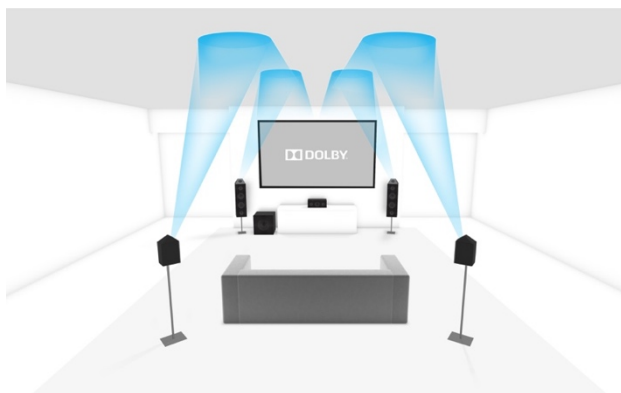
Figure 8: A traditional 5.1 speaker layout with five listener-level speakers and four Dolby Atmos enabled speakers (5.1.4).
