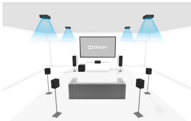
Figure 5: If you use overhead speakers, Dolby recommends using four or more.
